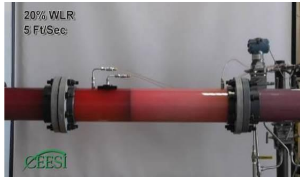
Fig 2. Cone meter 1.6 m/s, WLR_m 0.2.
