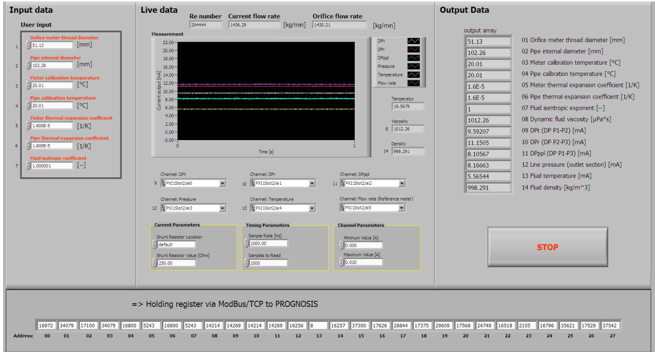
Figure 11 – Program interface (user interface) of the LabView program
