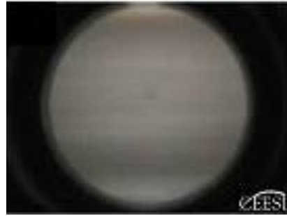
Fig 30b. Annular Mist Flow
