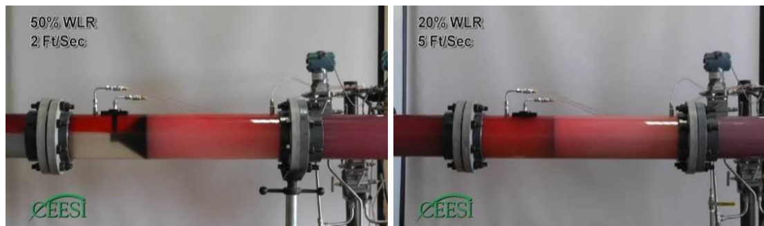
Fig 9. Cone meter, 0.6 m/s, \omega_m 0.5.
